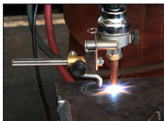
Small cutting circle (Ø30-200 mm)
