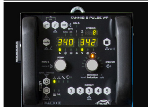
FANMIG 5 WP PULSE control panel
