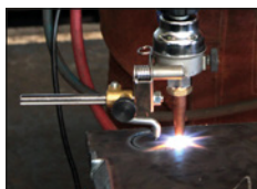
Small cutting circle (Ø30-200 mm)
