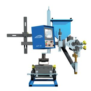
Control panel with a touch-sensitive display PLC fitted in for programming and parameters settings. This unit is equipped with internal memory that allows setting and restoring personal welding programs, current and welding voltage measurement, preliminary setup, voltage-current graph and linear energy transfer. Intuitive control system with an additional knob to set and correct all the most important operating parameters.
