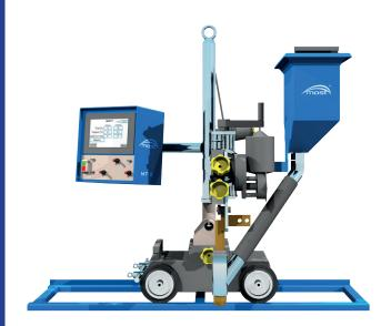
Standard version includes: tractor MOST MT-2, power feeder MOST Ponte-800c or 1000c, power-control wire 20m (2x95mm2) and earth wire 10 m (2x95mm2 – ring terminals), track section 2x1,5m, torch extension arm for fillet welds, swivel mast up to 50°, swivel head up to 60°, 360° head rotation around mast, vertical support L80mm, flux container 6L, laser indicator of welding axis.
